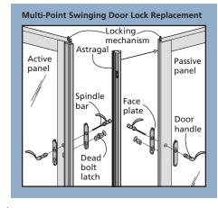
4. Unscrew and remove locking mechanism.
