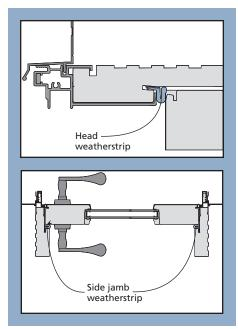
When replacing frame weatherstrip, if applicable, trim and overlap the new weatherstrip in the same way as the old weatherstrip.
