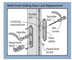
move the keeper up or down to align with the guide pin. Compare replacement handle set or lock to your existing hardware to make sure you have the correct new hardware. When removing screws and parts, keep track of their exact locations for reinstallation.
