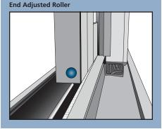
not present, or it is a (+), clockwise rotations will lower the panel, and counterclockwise rotations will raise the panel. Opposite adjustments apply to the (-) sign. Use a Phillips screwdriver for end adjusted rollers. Clockwise rotations will raise the panel, and counterclockwise rotations will lower the panel.
