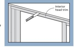
3. Remove the operating panel by sliding it away from the side jamb. Tilt the top of the panel to the interior, remove head track and lift up and over the sill track
