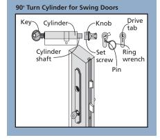
4. Hold the cylinder shaft in this position and remove the cylinder body from the door.
