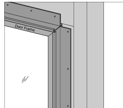
Fig. 4. Secure head extension jamb
