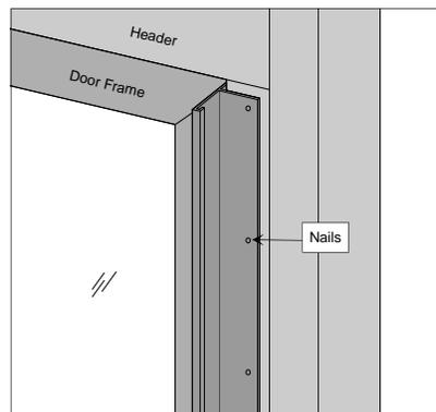
Fig. 3. Secure side extension jamb
