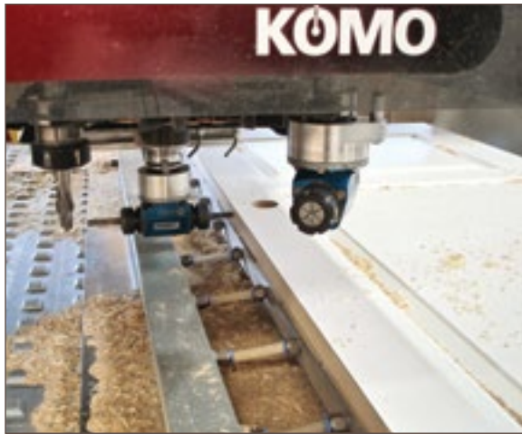
KOMO machinery routes the door contours and mortises the hinges and bores
