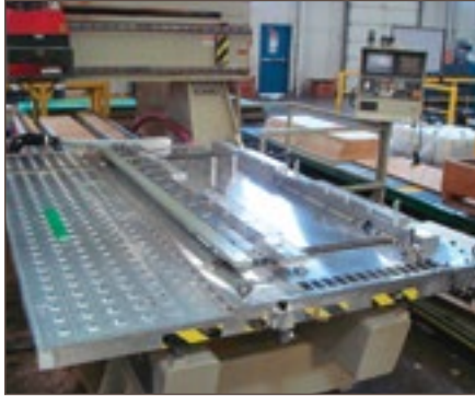
KOMO machinery routes the door contours and mortises the hinges and bores
