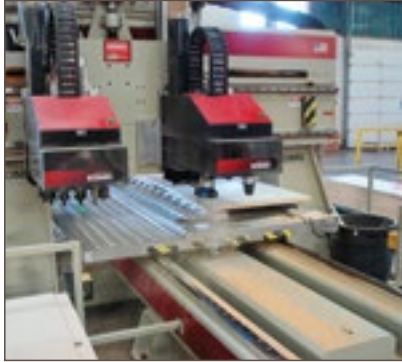
KOMO machinery routes the door contours and mortises the hinges and bores
