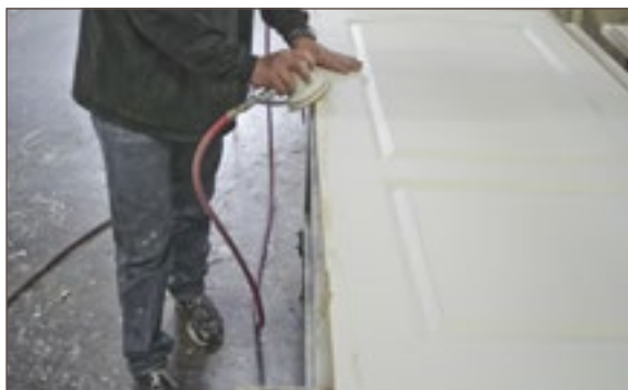
Routing, sanding and painting of the new door is done at the JELD-WEN plant
