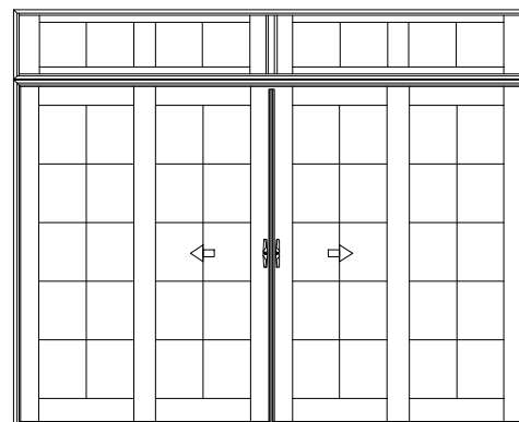
QUAD 2-PANEL (4-LITE) TRANSOM (WILL ALIGN WITH INTERLOCKS ON QUAD DOOR) AVAILABLE ON 10-0 & 12-0 WIDTHS ONLY
