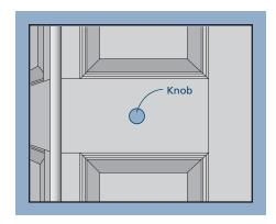
**Note!** Unless drilling the knob attachment hole close to an edge on a hollow core door, it will likely be in a hollow part of the door. This does not cause problems and the door material is sufficiently strong if the screw is snug but not over tightened.
