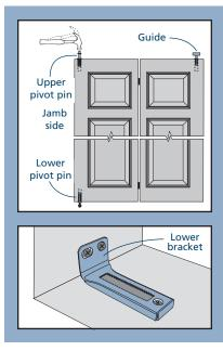
pre-drilled holes until snug. If installing four panels with two tracks, use a track bracket between the two ends in the center.
