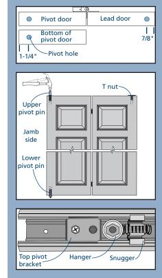
5. Secure the track to the head jamb with the provided #8 x 1" pan head screws through the pre-drilled holes. Move the top pivot bracket back toward the track end until it is 1/4" from the jamb and tighten the screw.
