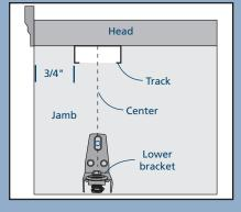
Unlock the track pivot latch by pulling the latch away from the jamb.With the door assembly folded, place the guide in the track and then
