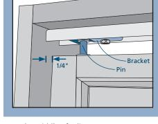
assemblies should be snug at the middle. If adjustments are necessary, door panels should be folded, in some cases removed, to gain access to the adjustment screws.
