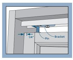
Two and four panel assemblies should have 1/4" clearance between the pivot doors and each jamb. Four panel assemblies should be snug at the middle.
