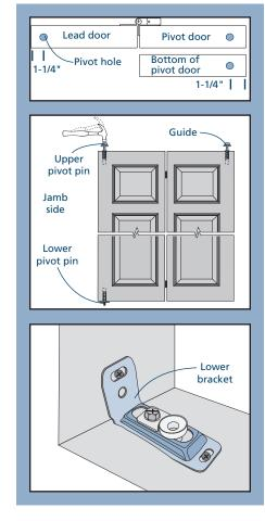
5. Place the upper pivot pin into the hole in the top pivot bracket and the guide pin into the track. Lift the assembly and place the lower pivot pin into the lower bracket. If installing a four door system, repeat for the other assembly. Check positioning and operation.
