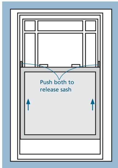
2. To check for device engagement, open window until device limits the window opening.
