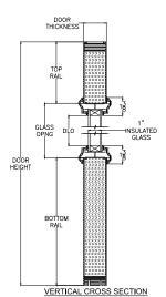
• Door Size = Book Size Before Prefit • Values in brackets [] are in millimeters • Wood grain = Mahogany • Door Cross-Section: • Moulding Profile = RGJS • Scale: 1/4\* = 1'-0\* • Panel Profile = n/a
