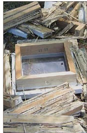
As you can see, after removing the window from its unprotected framework, the AuraLast Wood clearly withstood the harsh elements of wood rot and termite attack.
