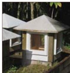
AuraLast Wood was put to the test for several years in a very harsh and humid environment. This test hut was built directly on top of a termite colony.
